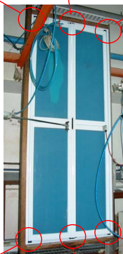
Photo 2: Close-up view of door components after endurance test.
